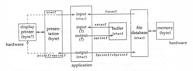
The Standard defines that field width and precision for %c, %s are counted by number of characters. In "single-byte character" world, a unit of character is equivalent to a unit of byte, 25 since 1 character is usually represented by 1 byte.
